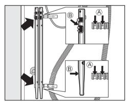
■ Secure the transit bars to the back of the washing machine. Make sure that holes (B) are fitted over retainers (A). The washing machine must not be moved without the transit bars in place.
